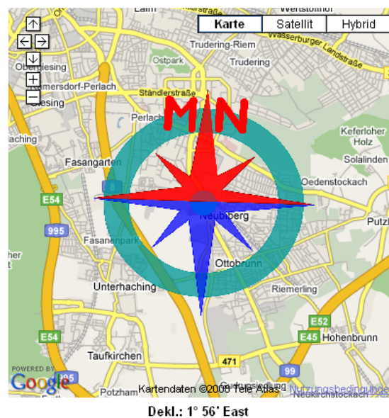
Figure 5-9: Declination as difference between geographic and magnetic North at the campus of the University of the Federal Armed Forces of Munich [123]
