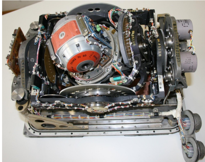
Figure 6-1: LITEF/Litton LN-3 platform INS system used in the F-104 G "Starfighter"
