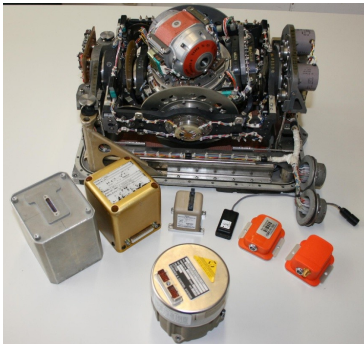
Figure 5-6: Evolution of inertial navigation measurement units over more than five decades. Sample of units from around 1960 to 2010
