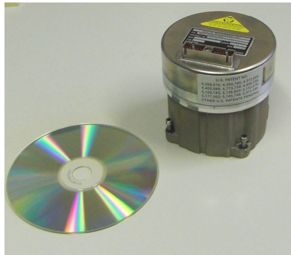
Figure 6-2: LITTON LN-200 strapdown IMU using Fiber-optical Gyroscopes (FOG)
