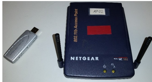
Figure 5-10: Typical WLAN equipment as used in the thesis
