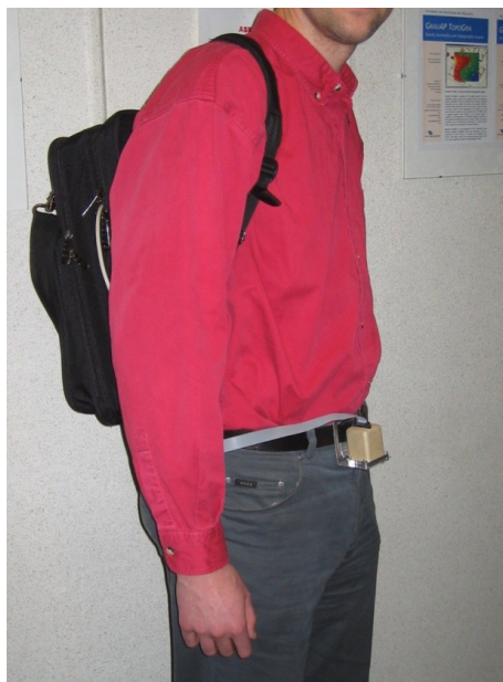
Figure 7-5: Sensor placement on the belt of the test person
