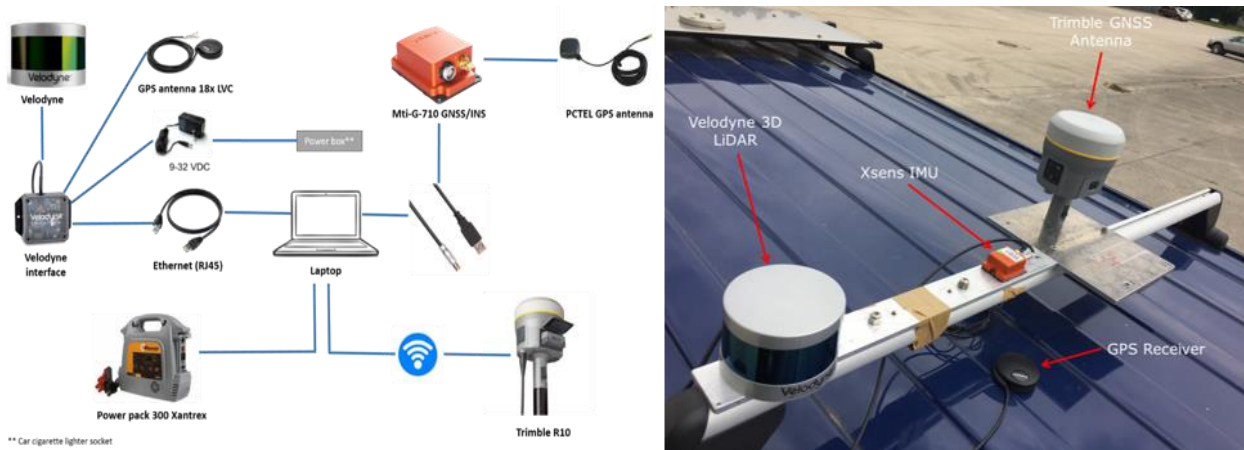
Figure 2. Scheme of the interface setup [left] and the mounting of the sensors [right]
