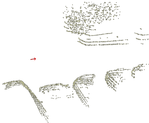
Figure 15. Point Clouds registration and LiDAR sensor displacement between consecutive measurements. Arrow's tail is the initial position, and the head is the final position.
