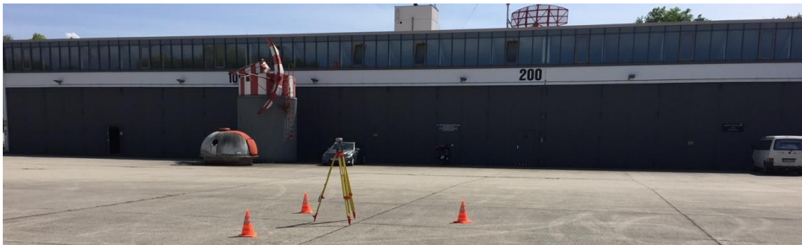
Figure 7. Scanning of the target with the reference system (MS60)
