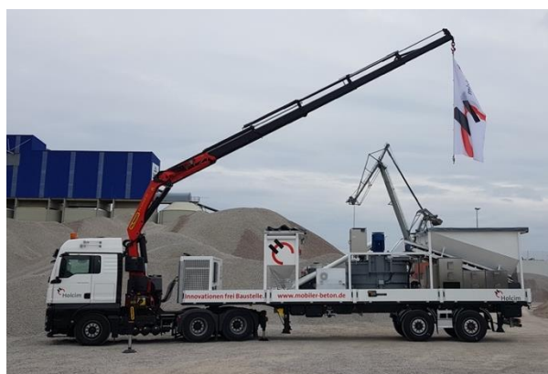
Figure 12. Truck-mounted concrete plant for ILC (courtesy: Björn Callsen).
