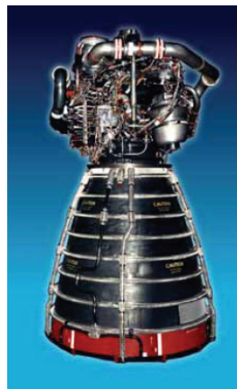
Figure 20: The Space Shuttle Main Engine (SSME), from [94]
