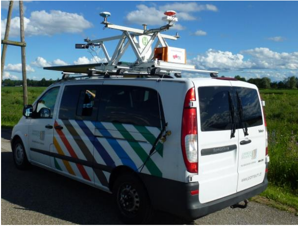
Figure 7: Measurement van with antenna setup on the roof and high-grade IMU
