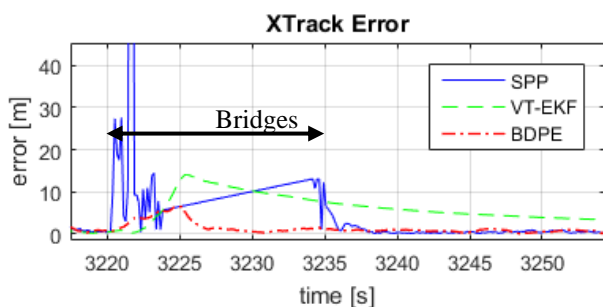
Figure 9. Cross-track error of under railway bridges
