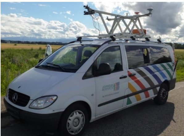
Figure 3. Measurement van with antenna setup on the roof and high-grade IMU (image: JR)
