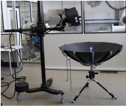
Figure 2. Surface accuracy measurement with optical measurement system.
