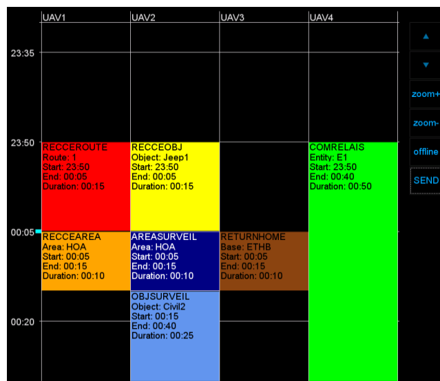
Figure 5-5: Overview screen of the alternative task-based guidance GUI
