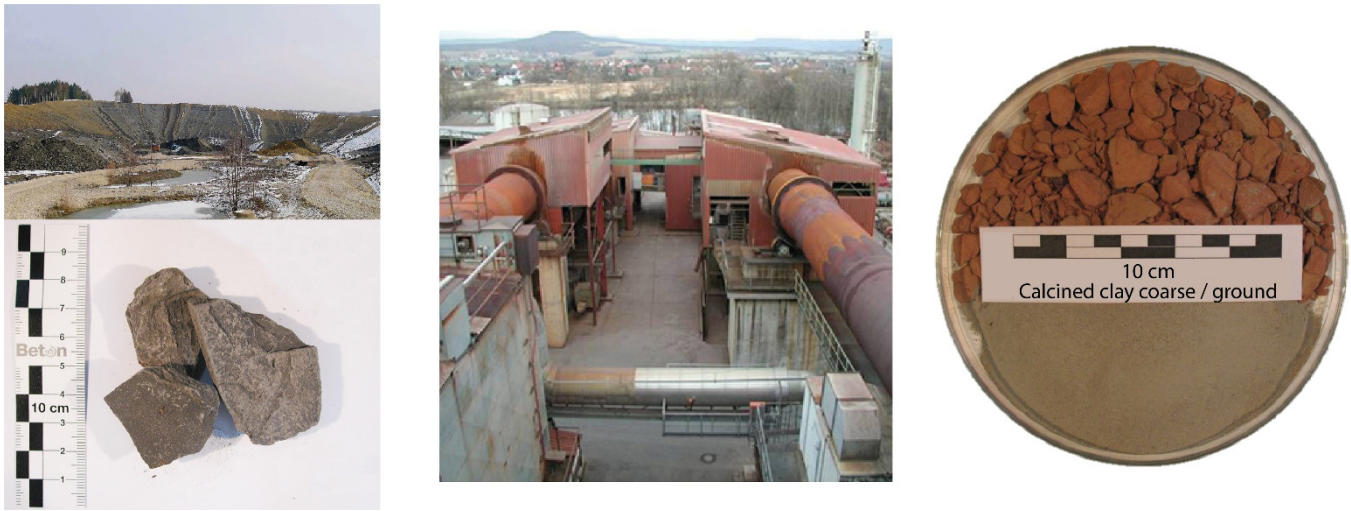
Figure 1 Exemplary production steps of clay-based SCM: Mining, pre-conditioning, calcination and processing (Source: Liapor GmbH & Co. KG, Pautzfeld).
