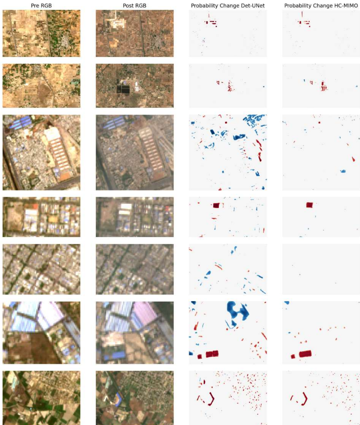
Figure 7. A quantitative change detection example for the New-Delhi area. From left to right: Pre-event RGB, post-event RGB, change in building probability for the naive baseline Det-UNet and the change in building probability for the best performing model HC-MIMO .
