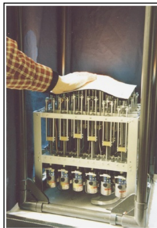
Figure 7. The Feelex I (developed in 1997). Source: Iwata, Yano, Nakaizumi, & Kawamura (2001), p. 471.
