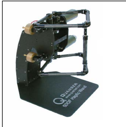
Figure 10. An example of a parallel-kinematic design: the Quanser 5-DOF Haptic Wand. Source: Quanser Industrials.
