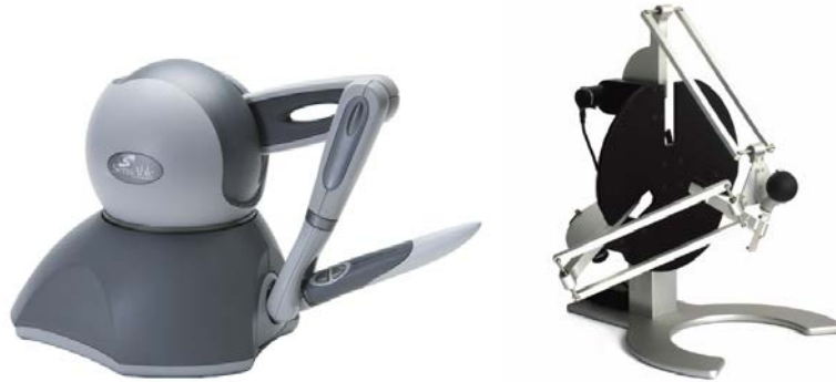
Figure 11. Two examples of impedance controlled haptic interfaces. The open-loop controlled PHANTOM Omni (left) and the closed-loop controlled delta.3 (right). Source: SensAble Technologies (left) and ForceDimension (right).
