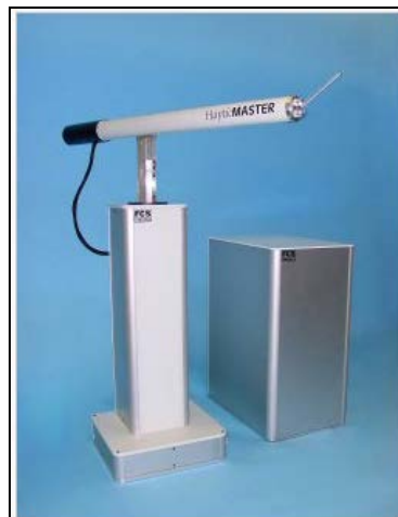
Figure 12. The admittance-controlled HapticMaster. Source: Van der Linde, et al. (2002), p.1.
