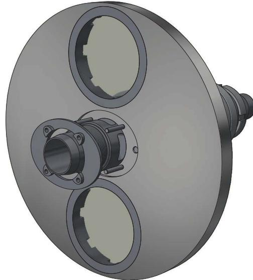
Figure 4.26: Inner disk with profiled disk spacer
