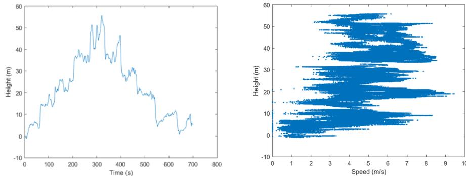
Figure 5 Altitude vs Time (LHS) and Velocity Profile (RHS) from Initial Flight of Quadrotor
