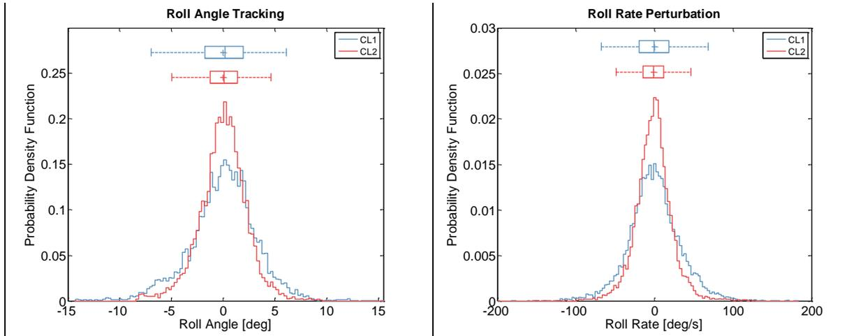
Figure 3 PDFs of Roll Angle and Rate With Different Stabilising Roll Control Systems
