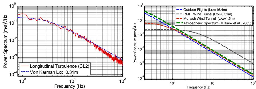
Figure 4 A Representative Spectrum in the RMIT Wind Tunnel LHS and Averaged Spectra RHS
