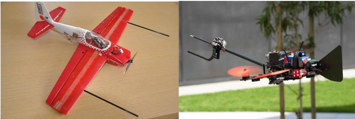
Figure 2 Slick 360 Aerobatic Model and Bespoke Quadrotor Craft Fitted with Pressure Probes.
