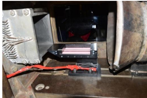
Figure 6: PSP measurement of cavity in the wind tunnel
