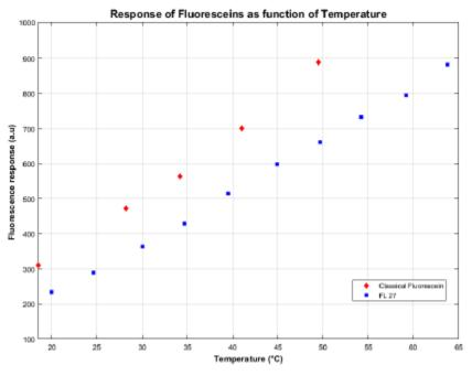
Figure 4: Response of Classical Fluorescein and FL27
