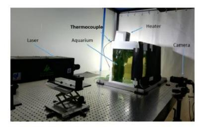
Figure 3: Calibration facility
