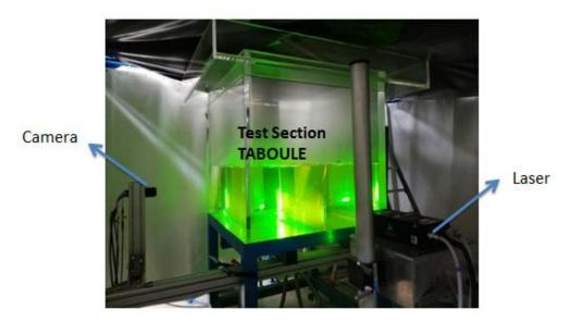
Figure 8: Test section of TABOULE
