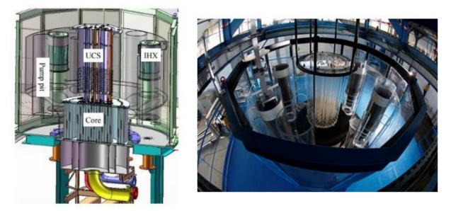
Figure 2: Left: Cross view of MICAS mock up; Right: Top view.
