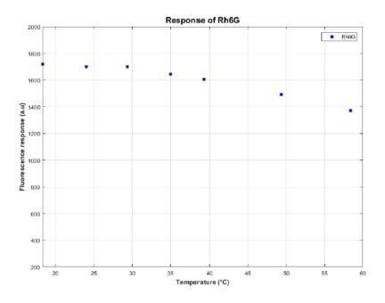
Figure 5: Response of Rh6G as function of temperature
