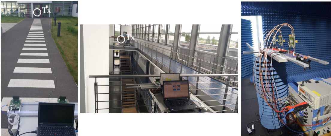
Figure 5.5: Three example measurement scenarios. Left: outdoor M = N = 2 scenario, FE 1, link distance between 10 m and 60 m. Center: indoor short-range backhaul M = N = 2 scenario, FE 1, distance of 15 m. Right: anechoic chamber M = N = 3 scenario, FE 2, distance of 5 m.
