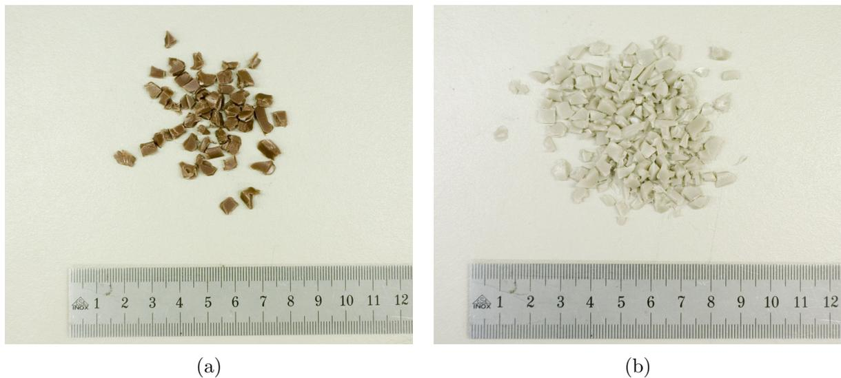
Figure 7.1: Typical plastic flakes produced by an industrial mill. (a) “Delrin 500NC010 Brown” labeled with the code “000101” (class 5). (b) “Hostaform C13031 White” labeled with the code “001010” (class 10).
