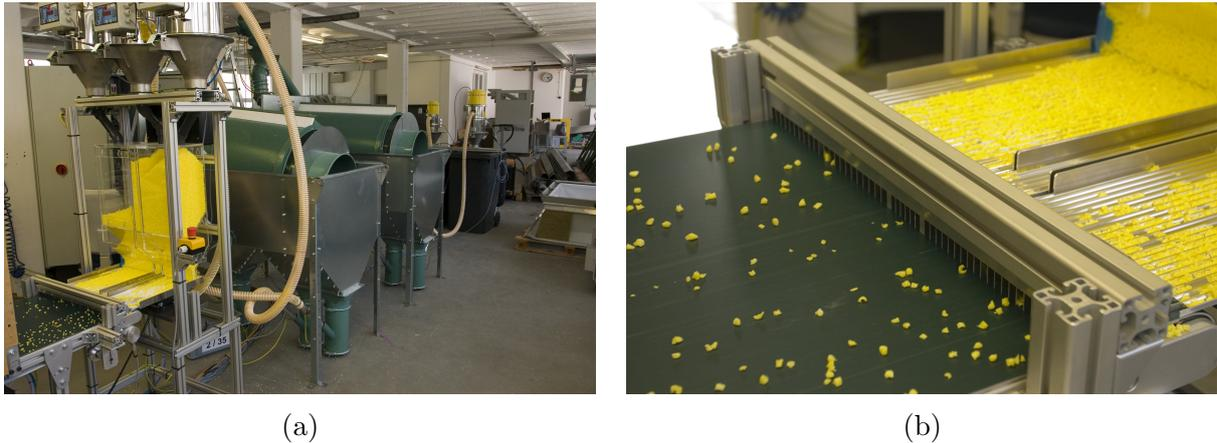
Figure 6.3: Singulation unit of the prototype system. (a) The system of filters to group plastic flakes by size can be seen in the background; containers with already grouped flakes and the shaker plate are in the foreground. (b) A close-up of the shaker plate with 50 grooves to separate plastic flakes in 50 parallel streams (channels) on the conveyor belt. Plastic flakes are all yellow for demonstration purposes.
