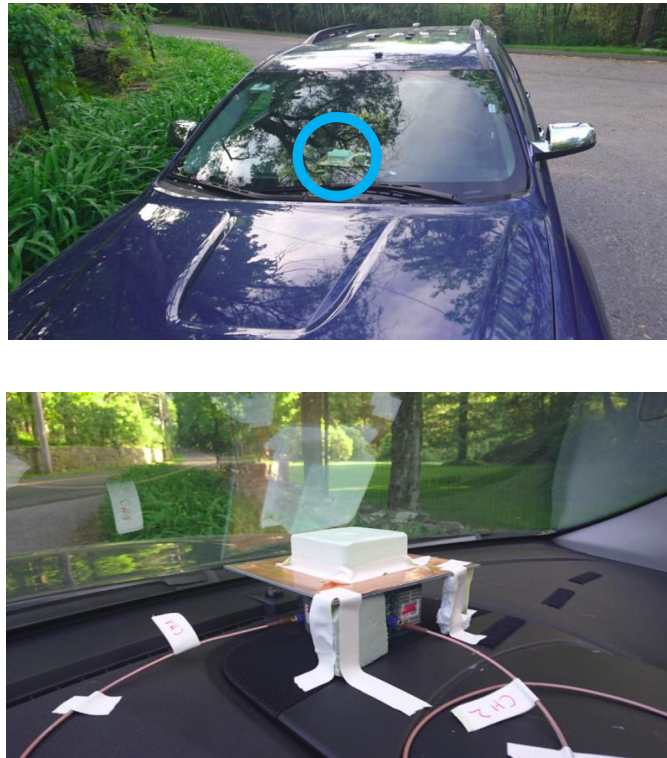
Figure 5.47: A micro-diversity antenna system mounted on the dashboard
