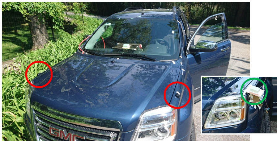
Figure 4.15: Antenna mounting positions of the measured antenna sets on the front fender(s). Big photograph: Two dislocated off-the-shelf commercial patch antennas (red circles). Image inset: Diversity antenna set (green circle) with two output signals on a single mounting position
