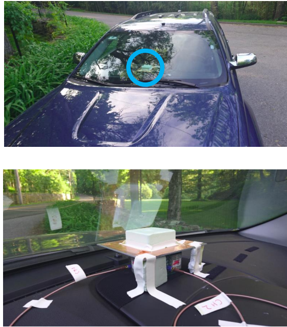
Figure 4.26: A micro-diversity antenna system mounted on the dashboard
