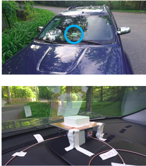
Figure 4.27: A micro-diversity antenna system mounted on the dashboard
