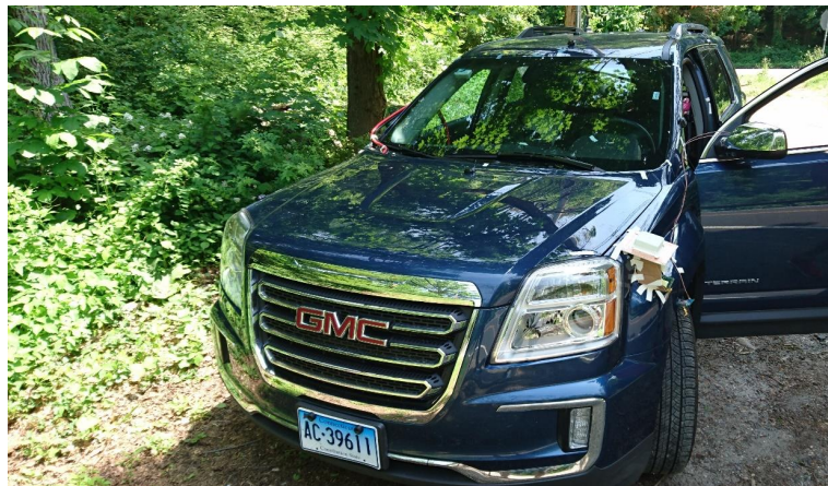
Figure 5.45: The micro-diversity antenna set composed of two loop antenna structures mounted on the front fender.
