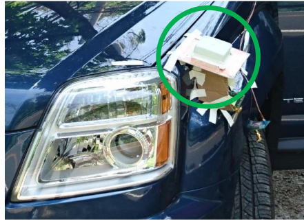
Figure 4.23: Micro-diversity antenna set (green circle) with two output signals on a single mounting position
