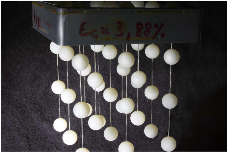
Figure 3.1: Photograph of one exemplary particle grid. Only the top two layers are fixed in all spatial directions. Every following layer is solely attached vertically, allowing the particle strings to move freely in a horizontal plane. Published in (Schlüter et al. 2021) and reprinted with permission.
