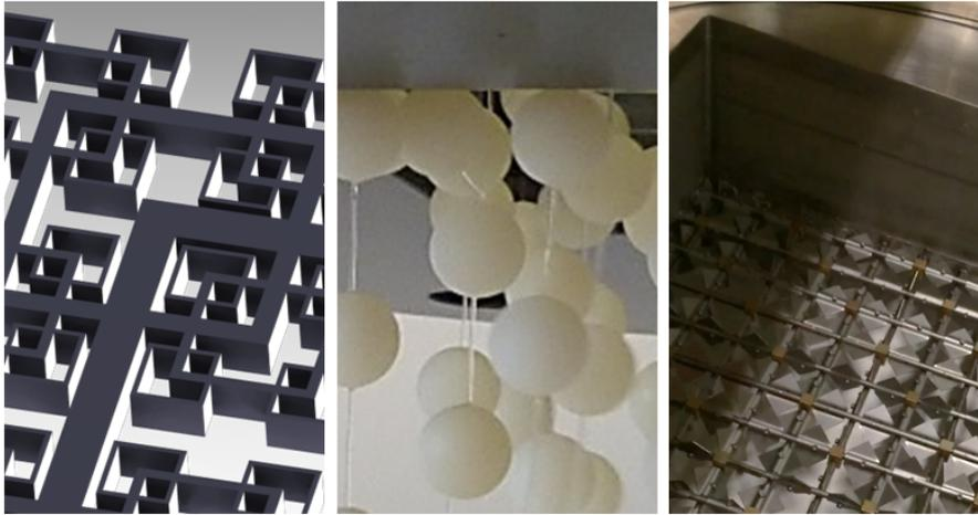
Figure 2.2: Comparison of the three different particle grids. From left to right the fractal grid, the free moving particle grid and the active grid.
