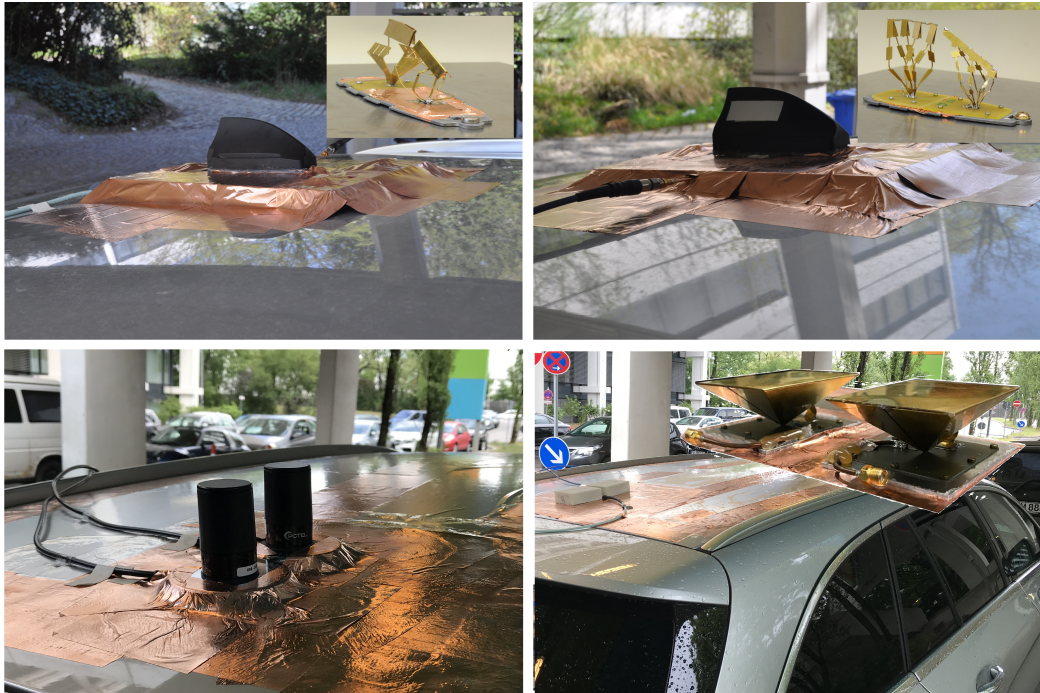
Figure 4.3: Roof antennas on test cars, antenna modules 1 and 2, reference antennas and flat Nefer antennas [43]
