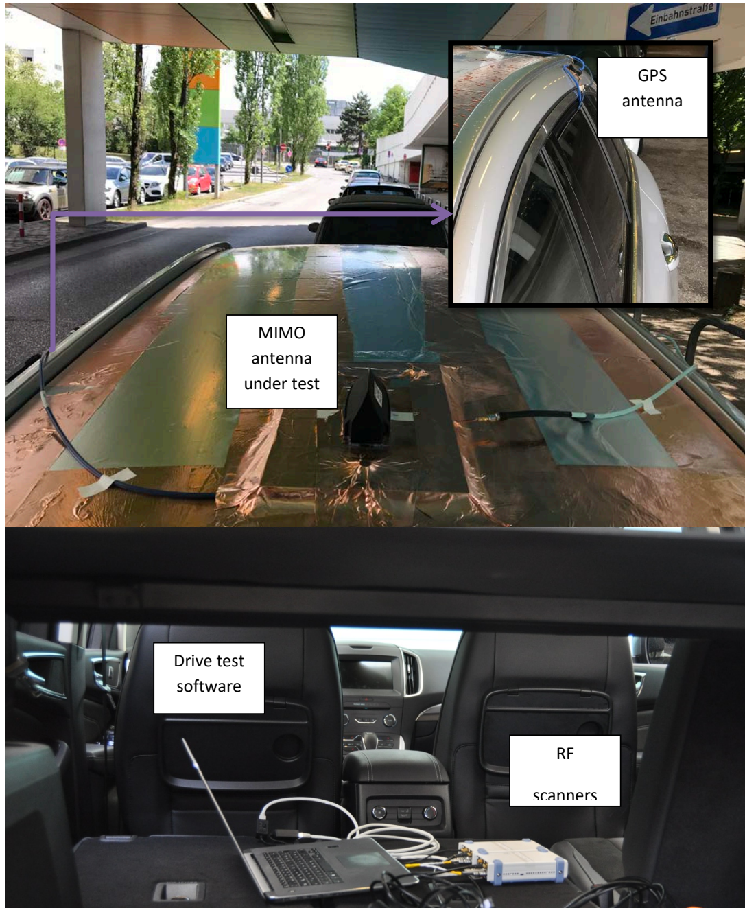
Figure 4.2: Drive test set up with the AUT, drive test software, RF scanners and the GPS antenna
