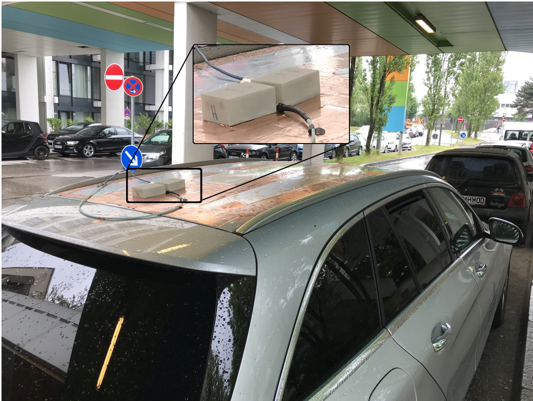
Figure 5.3: Two flat Nefer antennas in front of each other on the roof of the test vehicle
