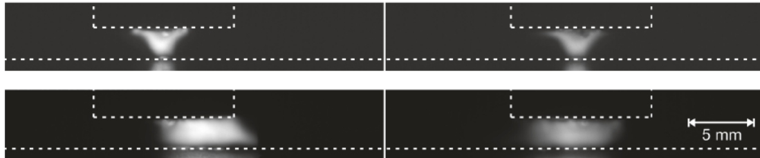
Figure 5. Stereo optical arc images during the magnetic field stud welding process (above: ignition of pilot arc; below: actual welding arc; left/right: images obtained with the left/right mirror of the stereo optical system). The dotted lines indicate the position of the stud and the work piece, respectively.
