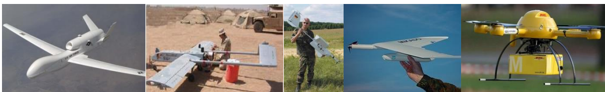
Abb. 4: UAV Beispiele: Global Hawk (HALE), Shadow 200 (TUAV), Aladin (Mini-UAV), Mikado (Micro-UAV), DHL-Paketcopter (VTOL-UAV) [Blom10, Rese14, Vach15]
