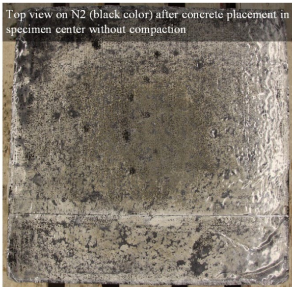
Fig. S1 – After the fresh concrete was placed on nonwoven N2 in the center of the specimen ( l/w/h = 600/600/200 mm) without vibration compaction, more cement paste was visible in the specimen center
