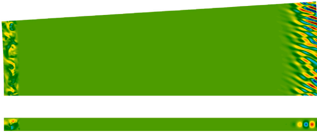
Fig. 4. Visualization of the volume force in Z-direction that is applied to the fluid field at the planes Z = 0 (top) and \phi = 0 (bottom) at one point in time during run C1.
