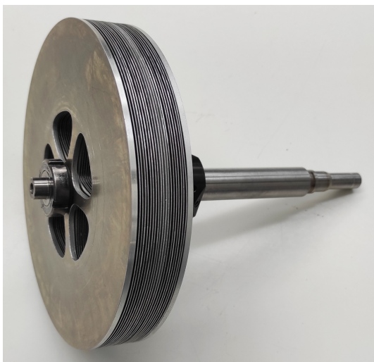
Figure 4.9: Rotor disk package mounted to the shaft.
