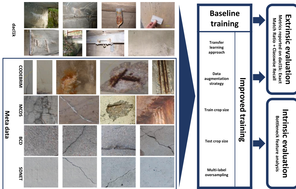
Fig. 1. Example images from the four analysed open-source datasets and our dacl1k dataset. Firstly, we train models based on results of previous research (Baseline training) and then apply five improvements to the training process (Improved training). Secondly, models are evaluated on datasets (Extrinsic) and the best model is further analysed (Intrinsic).
