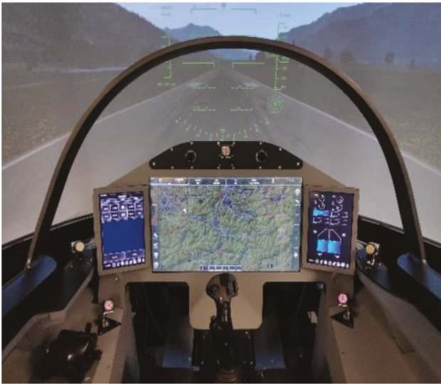
Figure 3. Cockpit simulation environment with integrated eye-tracking system.
