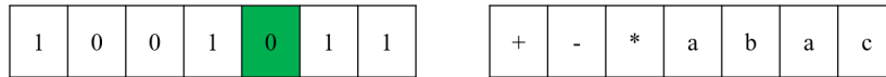
Figure 4.1: Scheme of the different genotype representations with binary (left) and string (right). A single allele is highlighted in green.
