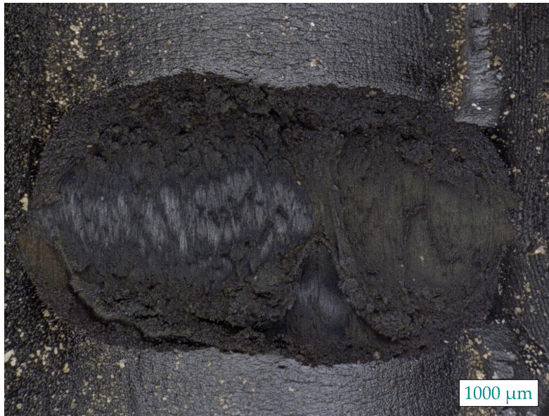
Figure 3.44 Crack tip structure after pre-ageing at 150 pphm ozone for 111 h under 30 % static strain.
