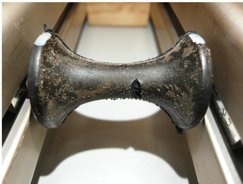
Figure 3.18 Visible cracks in hourglass sample after ageing 55 h at 150 ppm ozone concentration at 30 % strain.
