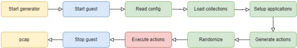
Fig. 2: Flowchart of the ForTrace Generator component
