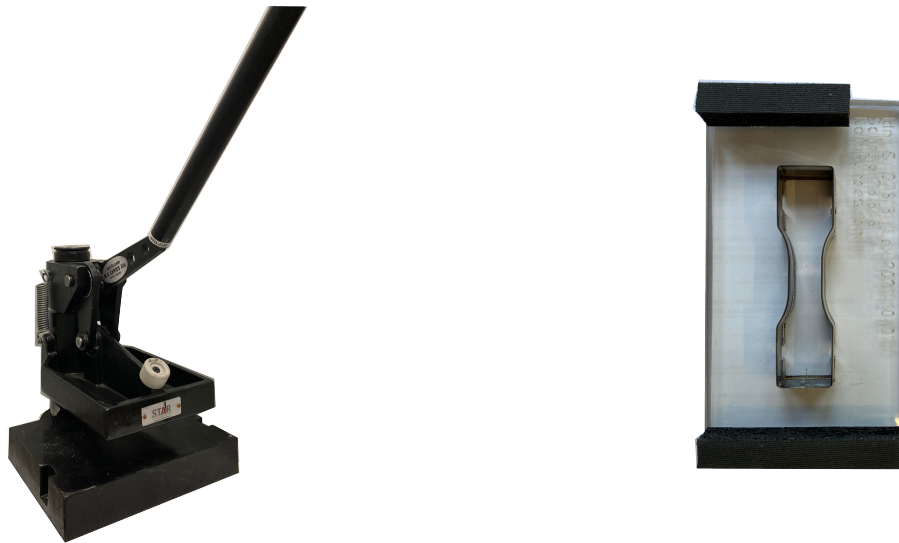
Figure 2.19.: Stamping machine setup from from Star cutting technology
