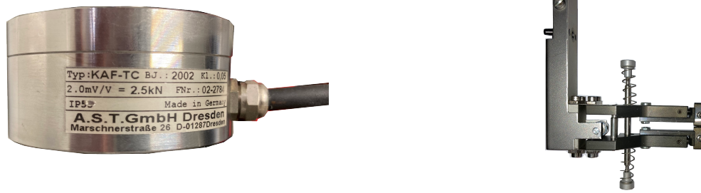
Figure 2.22.: Force Transducer from A.S.T GmbH (left); Displacement Transducer from ZwickRoell GmbH & Co. KG, article number 024895 (right))
