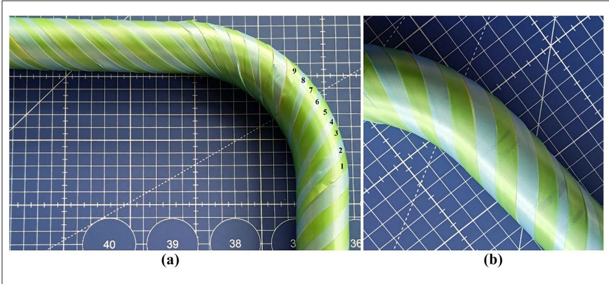
**Figure 15.** Winding a layer of rovings/tapes on a shaped frame (input values correspond to Table 5: major radius of torus  $R = 102[mm]$ , minor radius  $r = 18[mm]$ , winding angle  $\alpha = 45^\circ$ ). (a) Several rovings/tapes according to parameters of the toroidal part (nine, Table 5), (b) Detail of overlaps on the toroidal part.
