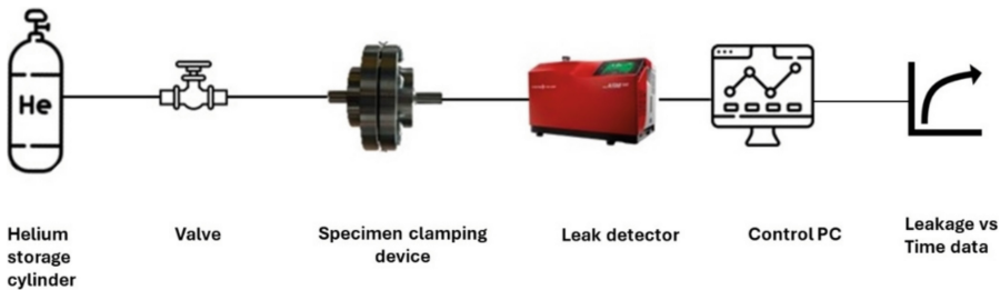
Fig. 10. Schematic diagram showing the inhouse permeation test set up.
