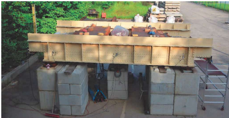
Figure 2: Test setup of riveted bridge
