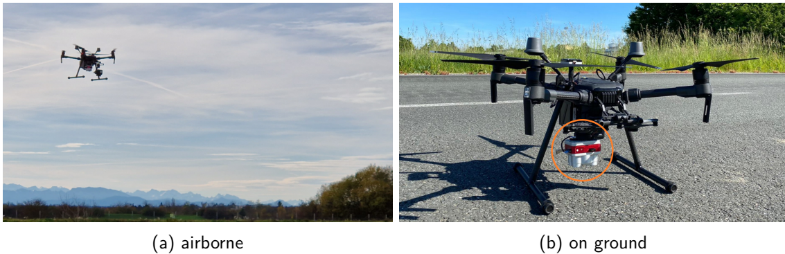
Figure 1.1: UAV with multispectral sensor payloads. The left image shows an airborne UAV equipped with multiple multispectral sensors, while the right image shows the same UAV on the ground with a single downward-facing multispectral sensor, providing six different spectral bands (annotated with an orange circle).
