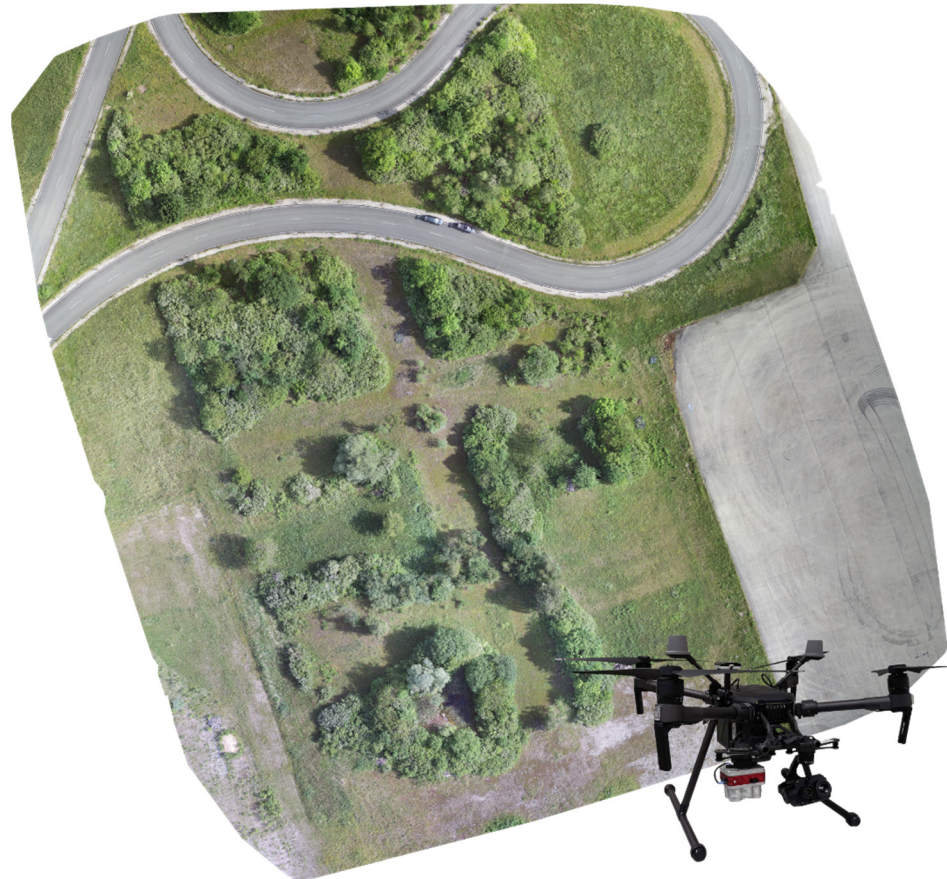
Figure 2. The visual orthophoto that was used to generate the visual bands of MUCAD. The setup utilized for taking the raw images was composed of a DJI Zenmuse XT2 and a MicaSense Altum mounted on a Matrice 210 RTK V2.
