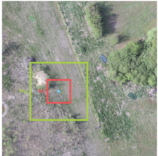
Figure 3. The dual window defining the neighborhood of pixels for the pixel under test (blue). The neighborhood consists only of pixels that are inside the outer window (green) but outside the inner window (red).
