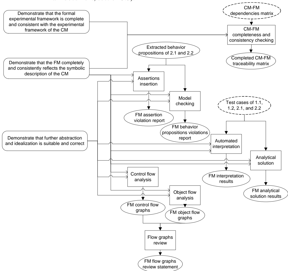
Figure 10: Dependencies between the objectives, techniques, inputs, and outputs of V&V sub-phase 3.2
