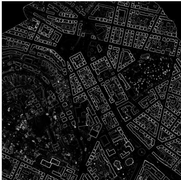
Figure 4.14: Local Range Variation ( LRV ) image which highlights height jumps
