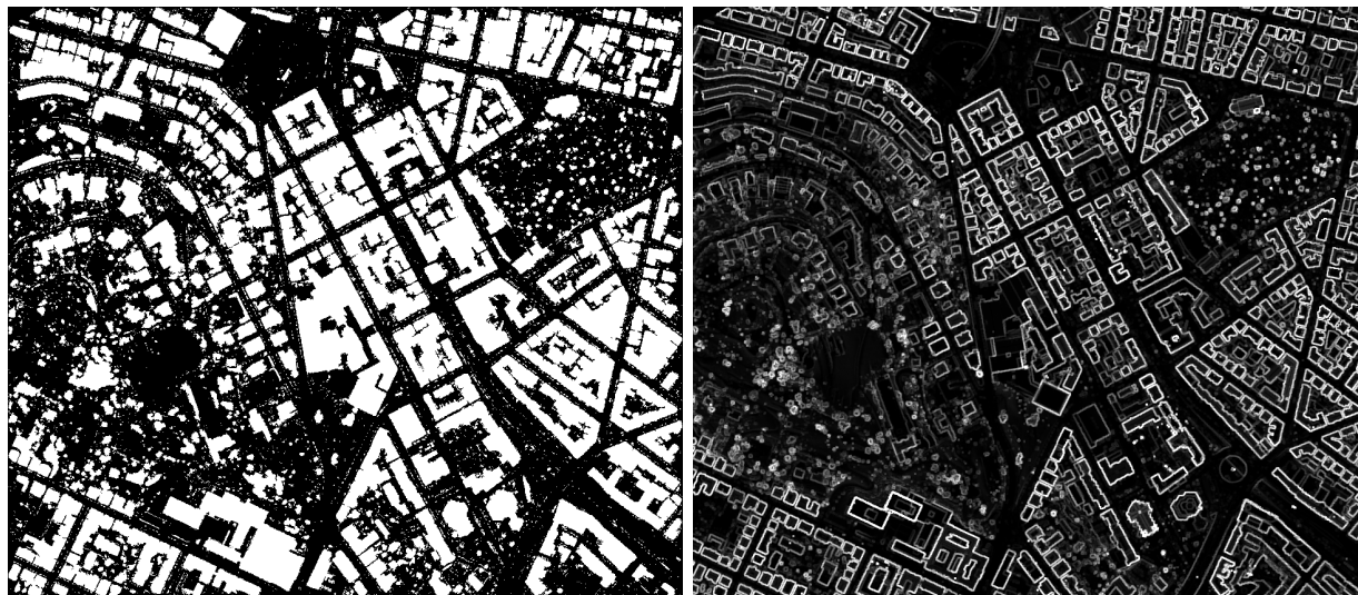
(a) Non-ground regions after final iteration – in this hilly area the number of iterations is 9
