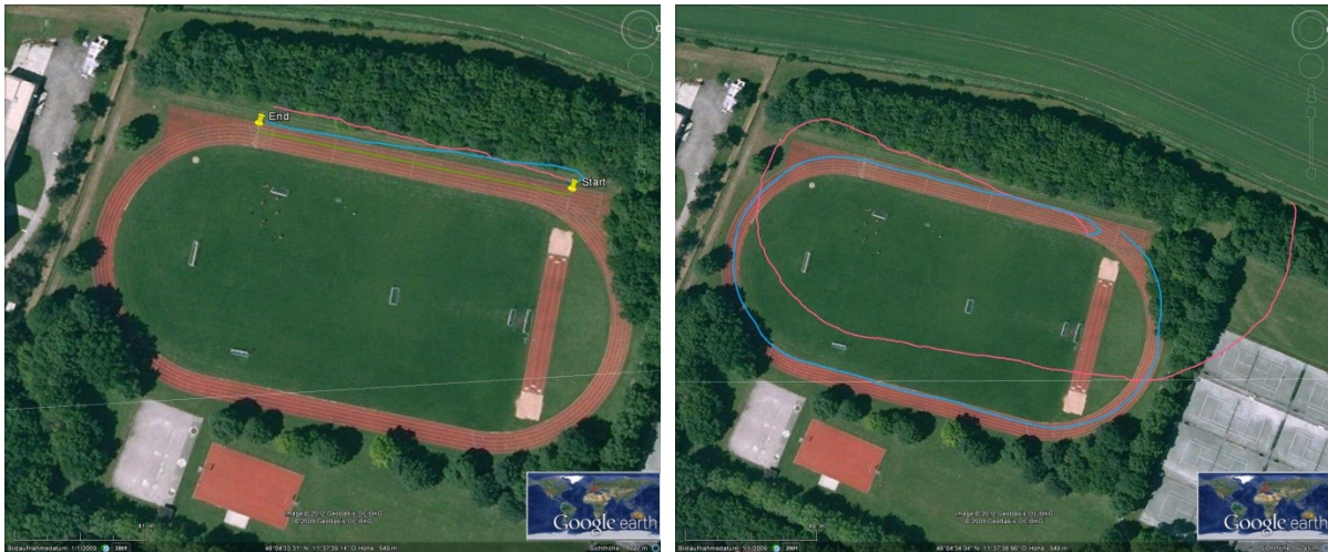
Figure 3-53: Test walks with the LG Optimus black 3D. The blue line is the tracked measured by the GPS receiver and the pink track is the one computed by dead reckoning.
