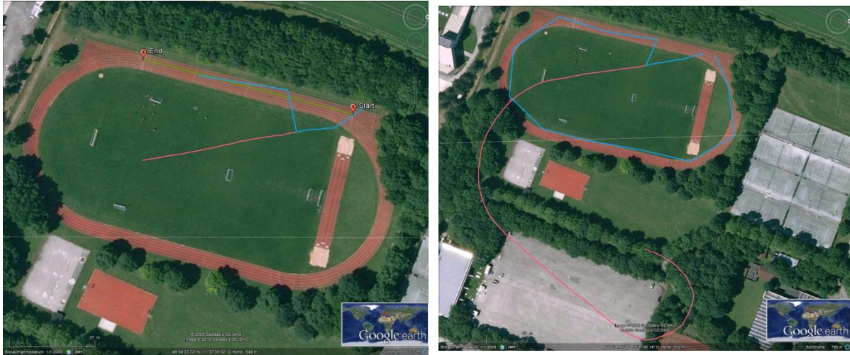
Figure 3-51: Test walks with the Samsung Galaxy SII. The blue line is the track measured by the GPS receiver and the pink track is the one computed by dead reckoning
