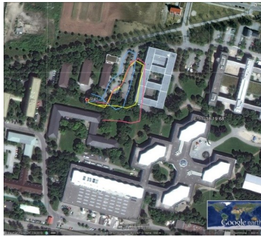
Figure 3-69: Measured track during walk 5 of the Samsung Galaxy. The map on the right side depicts the GPS track in blue, the dead reckoning track in pink and the Kalman filtered track in yellow.
