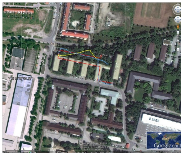
Figure 3-73: Combined outdoor-indoor track of the Samsung Galaxy. The red line indicates the true path through the building, the blue track depicts the GPS estimated position and the yellow line the filtered dead reckoning position.
