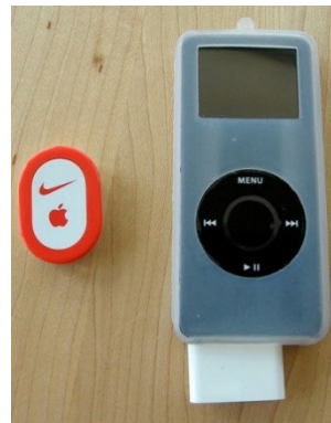
Figure 2-16: The iPod Nano with attached receiver (right) and the accelerometer (left) which is placed in the left training shoe (photo from wikipedia.de)
