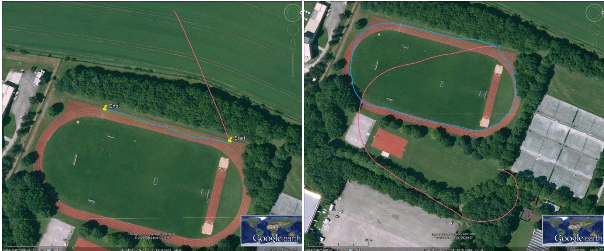
Figure 3-52: Test walks with the Google Nexus. The blue line is the track measured by the GPS receiver and the pink track is the one computed by dead reckoning.
