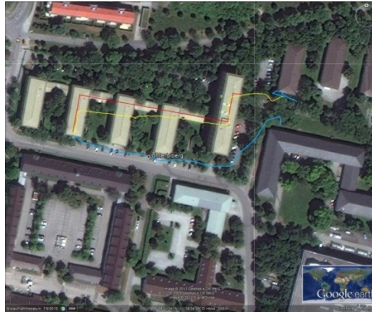
Figure 3-71: Combined outdoor-indoor track of the LG Optimus. The red line indicates the true path through the building, the blue track depicts the GPS estimated position and the yellow line the filtered dead reckoning position.
