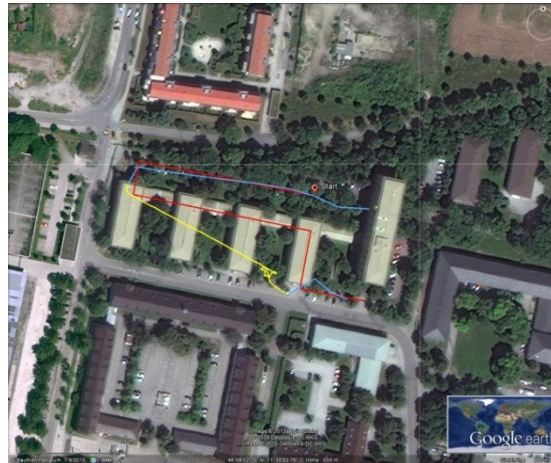
Figure 3-72: Combined outdoor-indoor track of the Google Nexus. The red line indicates the true path through the building, the blue track depicts the GPS estimated position and the yellow line the filtered dead reckoning position.
