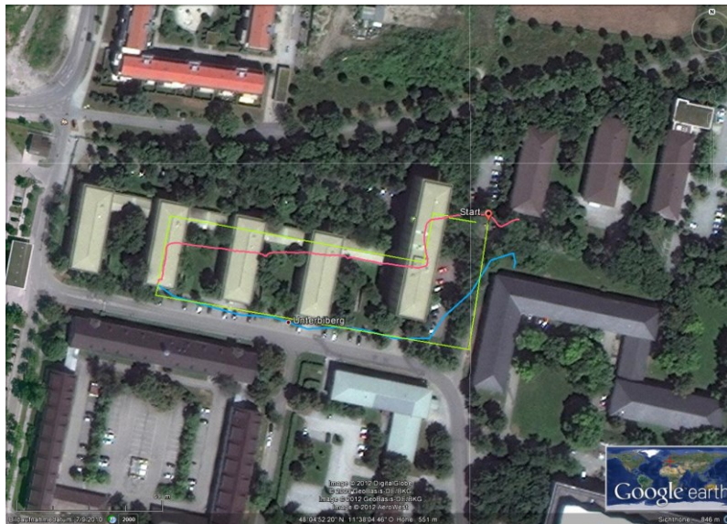
Figure 3-62: Combination of outdoor and indoor environment walked with the LG Optimus. Blue indicates the GPS computed track, pink the dead reckoning track and the green line the true track walked.
