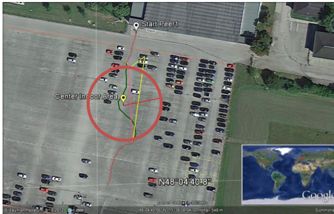
Figure 3-76: On the left side the GPS estimated track of peer 1 in green, the dead reckoning only track in pink and the filtered track in yellow. On the right side the position error of dead reckoning and filtered track in km. One peer was present in this scenario.
