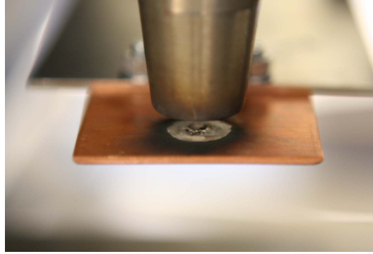
Figure 5.5: Nozzle of gas metal arc with donut cathode.
