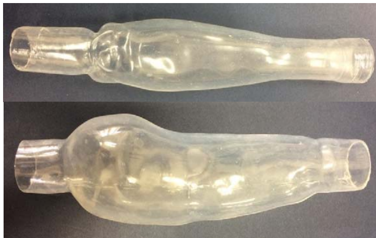
Figure 3: Aorta models used during the tests. Top panel: aneurismatic aorta 48mm; bottom panel: aneurismatic aorta 64mm
