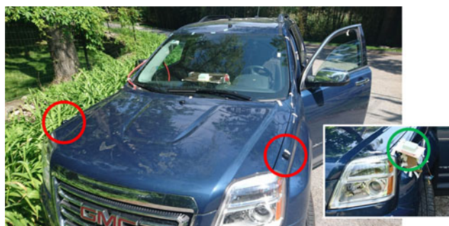
Fig. 10. Antenna mounting positions of the measured antenna sets on the front fender(s). Big photograph: two dislocated off-the-shelf patch antennas (red circles). Image inset: diversity antenna set (green circle) consisting of two loop antenna structures with two output signals on a single mounting position.
