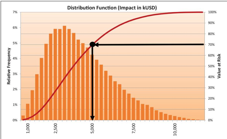
**Figure 4. Probability density distribution function showing probable project cost with Value at Risk information**
