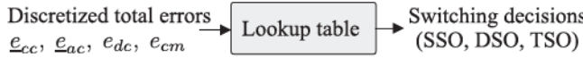
Fig. 14. Lookup table is used to obtain optimal switching decisions based on discretized total errors.
