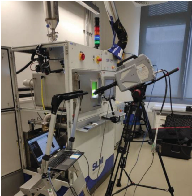
Fig. 3 SLM@125HL and high-speed camera setup
