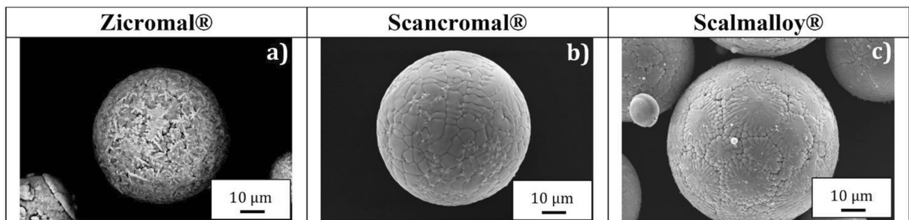
Fig. 1 SEM (BSD) pictures of (a) Zicromal®, (b) Scancromal® and (c) Scalmalloy® powder
