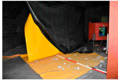
Figure 3. Areas for collection of secondary debris (left), curtain construction to stop the secondary debris (right).
