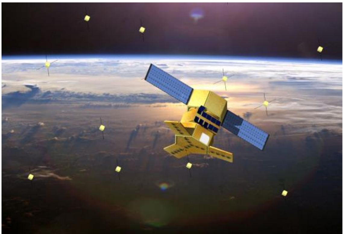
Figure 1-2 An artist's visualization of the proposed satellite concept showing the larger chief satellite with the correlator antenna in Y-configuration and the other Cubesats (deputies) in close proximity.
