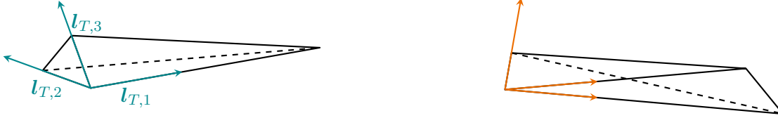
Figure 2.3: Comparison of two anisotropic tetrahedra, with regular vertex property (left) and without regular vertex property (right).
