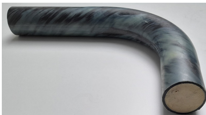
Figure 15. Example of the curved part of polymer composite frame with the following parameters: major radius R = 102.5 [mm], minor radius r = 17.5 [mm], width of roving d = 5 [mm]. The non-load-bearing polyurethane frame is visible in the vertical section (light colour of the cross-section).
