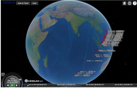
FIGURE 6.25: Fragment debris orbit visualization 1 hour after the collision event.
