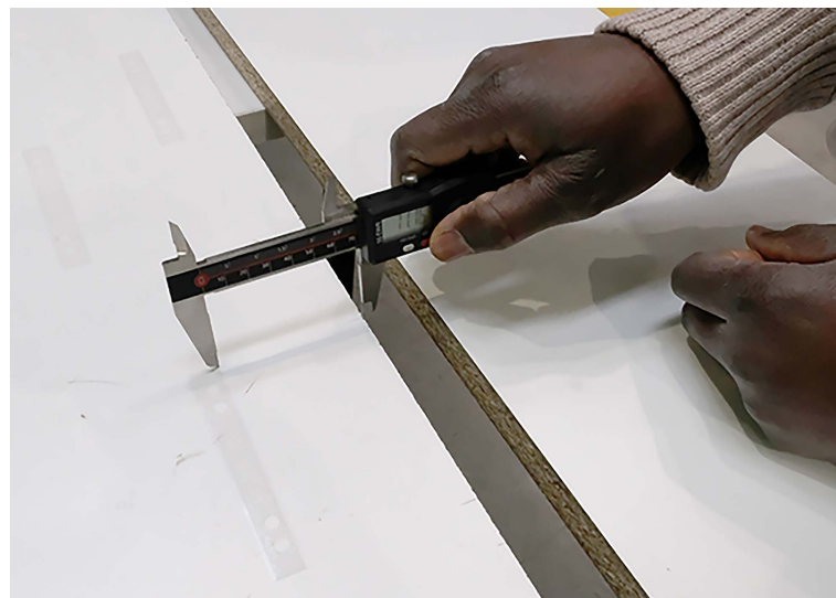
Figure 8. Evaluation of the angle of misalignment using a sliding caliper.
